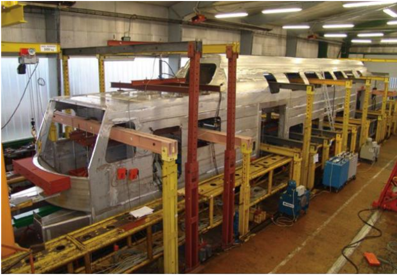
Figure 4: Full-size railcar body set up for static testing
