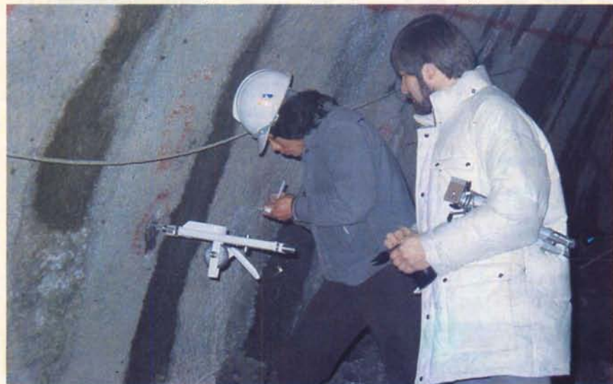
Accurate measurement has led to the realisation that initial rapid support is not always the best policy. In certain circumstances, initial movement should be allowed.
