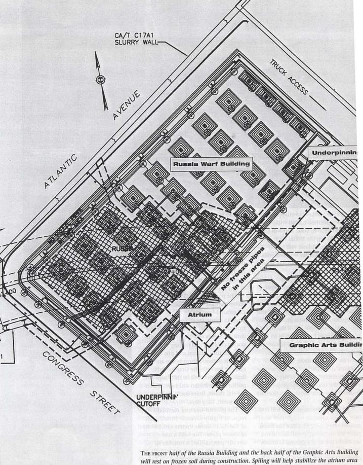
will rest on frozen soil during construction. Spiling will help stabilize the atrium area between the two buildings.
