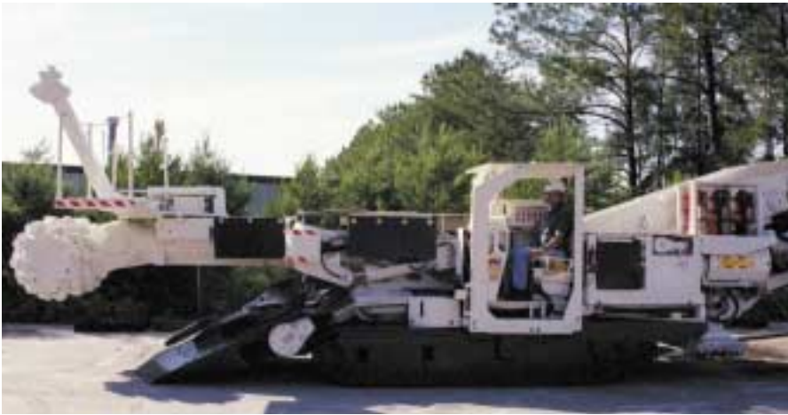
The Voest Alpine AM 75 used on the project prior to delivery on site
