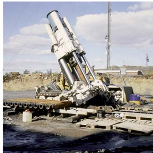
Figure 1b: Raise Boring Machine for inclined shaft at a copper mine - Bolivia 1986
